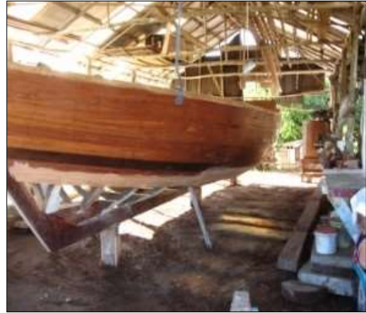
Traditional Sarteneja fishing boat being constructed – a craft past from father to son
